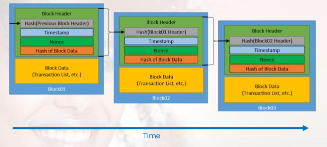
Blocks are <u>chained together</u> through each block <u>containing the hash digest of the previous block's</u> header, thus forming the block chain
